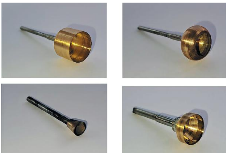
Figure 3 – General view and shapes of hollow thin-walled heads.
