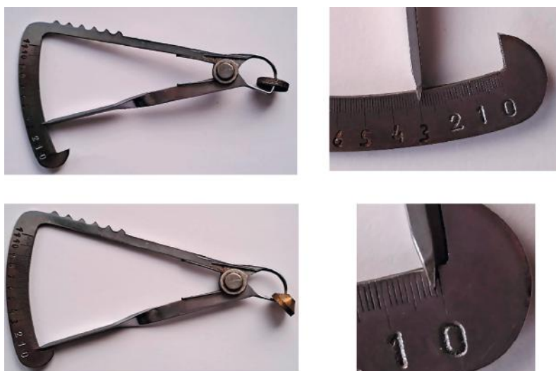
Figure 5 – Dental micrometer with test specimens.
